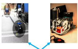
Security: the winch is equipped with an anti- roll back mechanism which prevents the wheelchair from moving back when it is stopped on the ramp.
