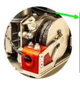
**Safety:** the winch is equipped with anti roll-back mechanism that prevents the wheelchair to back up when it is stopped on the ramp.
