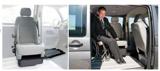
It allows you to move the driver seat backwards, rotate it and adjust it in height to bring the driver seat next to the wheelchair.
