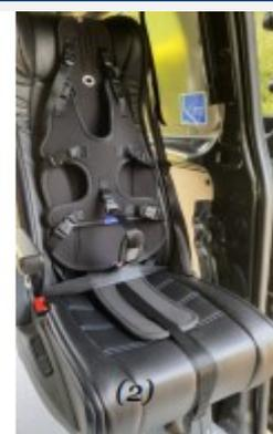
**Important information:** The standard emergency evacuation system is reachable behind the seat or by the trunk. You only need to click on the 2 red buttons at the same time and the person can leave the car together with the harness.
